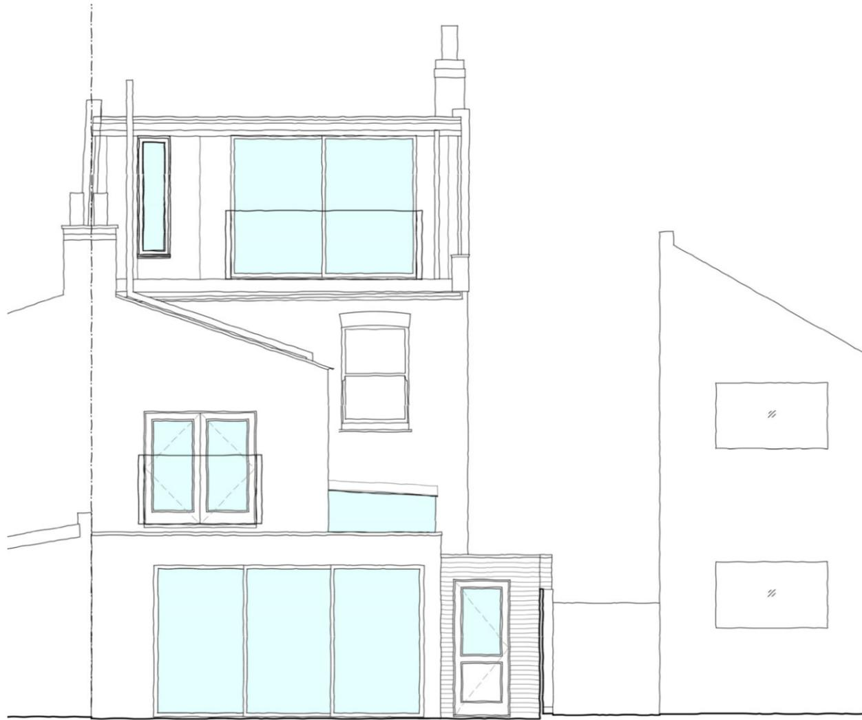
The ground floor side extension is set back from the main frontage and creates a much needed utility room. The rear infill extension includes a large structural glass rooflight and minimal frame sliding glass doors.
