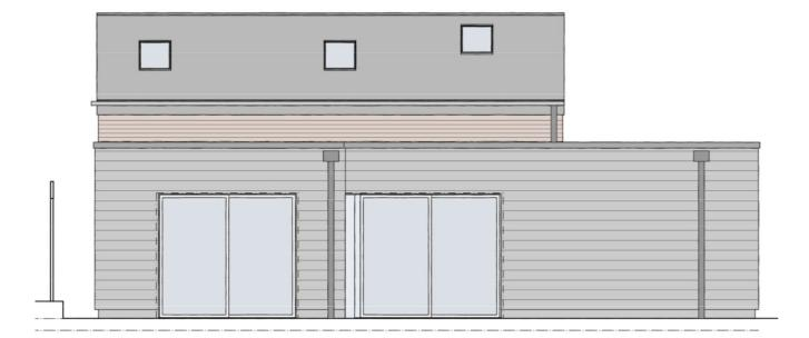
The building design is intended as a contemporary interpretation of the local building forms, with modern, robust materials such as fibre cement board cladding, London stock brickwork, slate and sedum roofs.
